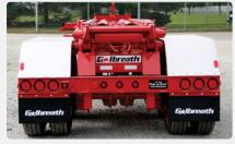
"Plug n' Play" wiring system eliminates crossed wires, loose connections, corrosion and splices; allows for simple light replacement.
