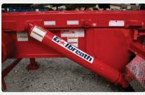
2 cylinders are mounted on the outside of the rails to provide stability when loading heavy boxes.
