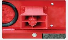
The hoist-up alarm is a standard safety feature. When hoist is raised, alarm will sound, warning of hoist and container movement.
