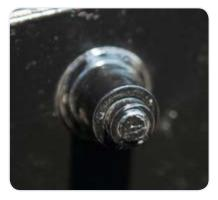
Hoist frames are huck bolted to chassis, providing unmatched strength and durability (factory mount only)
