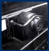
Rear skid plate with outboard supported rollers
