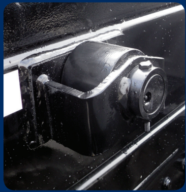
Rear skid plate with outboard supported rollers
