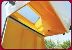
LIFELINER® HOPPER SYSTEM The LifeLiner® system is a specially designed hopper liner and finish system that greatly improves the life, durability, and functionality of a sweeper hopper.
