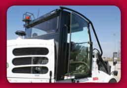
LIMB GUARD Heavy-duty guards surround cab and protect sweeper by guiding lowhanging tree limbs up and over the Pelican. Available in right hand, left hand, or dual configuration.
