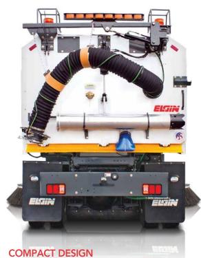
The sweeper mounts on conventional or cab-over chassis with short wheelbases, enabling a tight turning radius for better reach in cul-de-sac sweeping, and greater maneuverability around tight corners. The standard auto pickup in reverse allows for quick change of sweeping locations.
